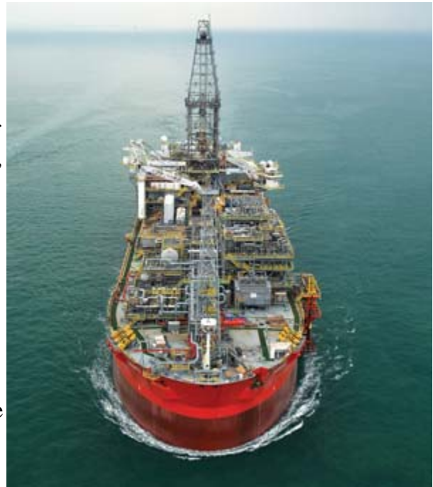
WFM designed and built another deck to support the drilling structure on the FDPSO. (Image courtesy of William Jacob Management Inc.)
